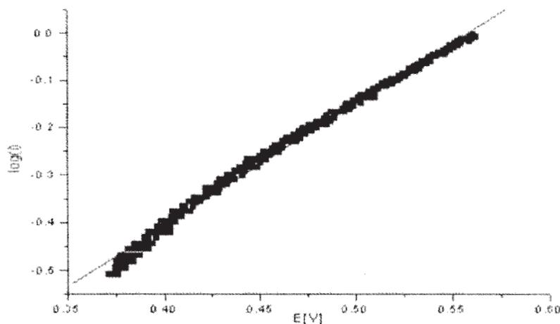
Fig. 4. Tafel plot of cyclic voltametry data
