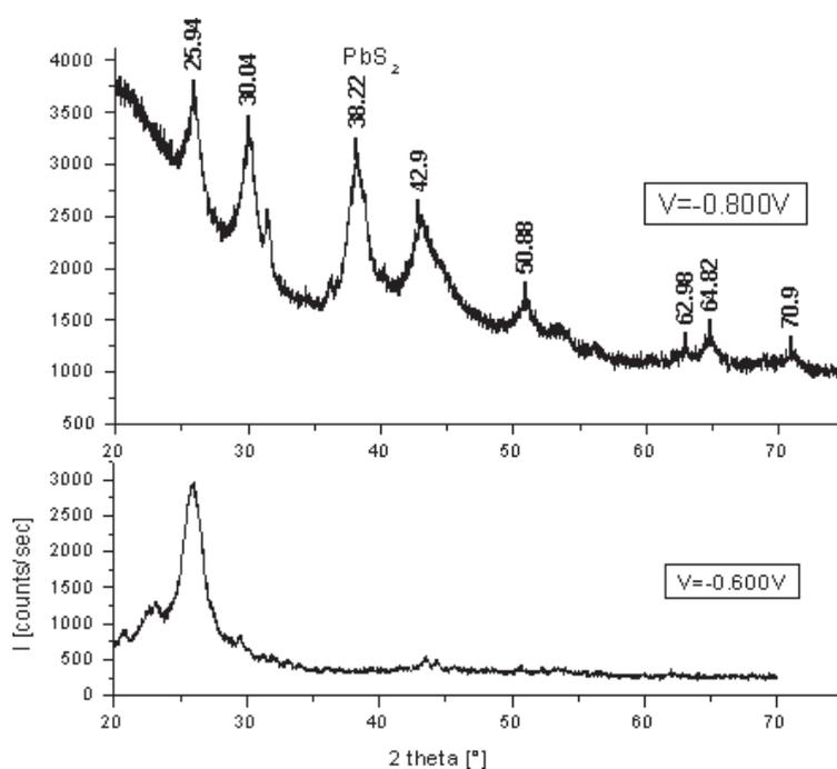
**Fig. 3.** XRD with a  $1^\circ$  glancing angle of: a) thin film anodised at 0.600 V b) thin film anodised at 0.800 V
