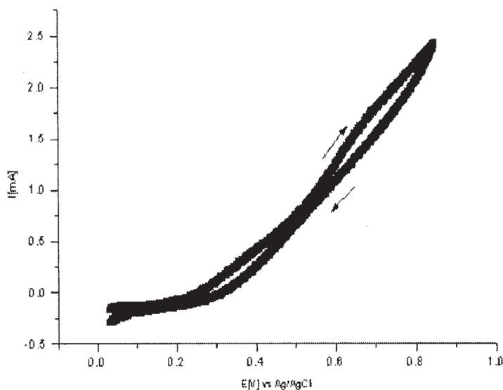
**Fig.1.** Cyclic voltammetry of partially anodised lead film, from 0.1 to 1 V, at 50 mV/s.
