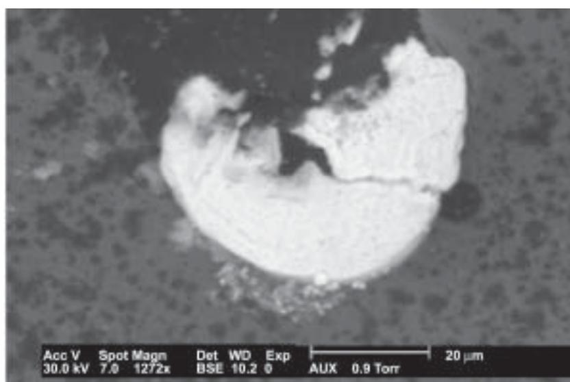
**Fig. 2.** Ambient SEM micrograph of PbS thin film.
