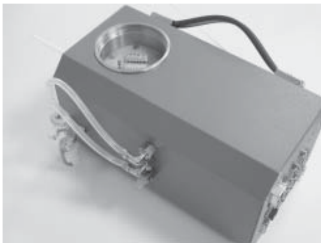
Figure 1: Image of the portable Electronic Nose developed at IMM-CNR - Lecce (Italy).
