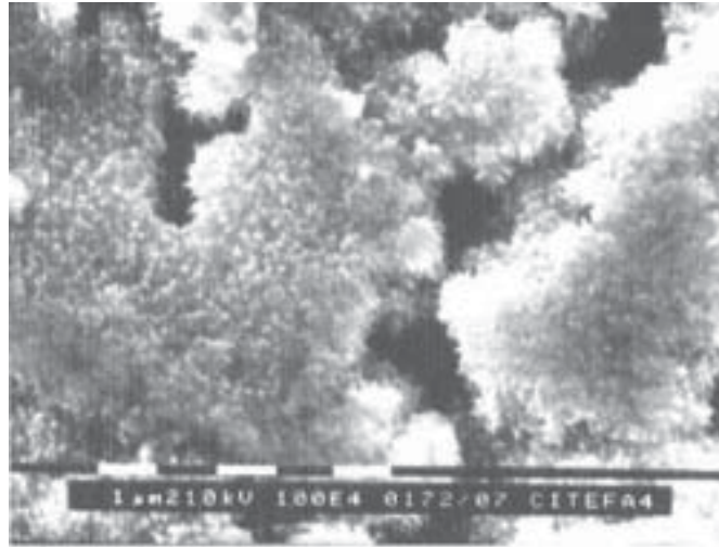
Figure 4: SEM micrograph of a Te film exposed to humid atmosphere for 15 days ( M = 10000x ).
