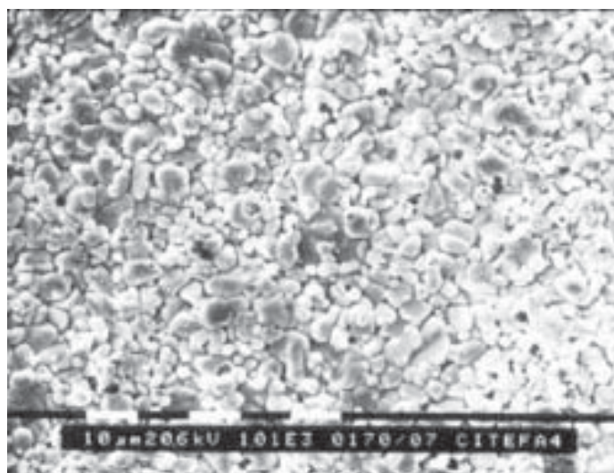
Figure 2: SEM micrograph ( M = 1000x ) of a Te film after being exposed to air for five days.
