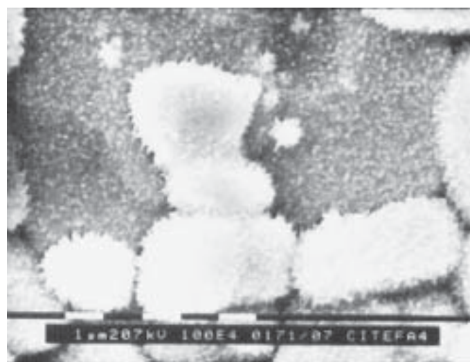
Figure 3: SEM micrograph of a magnified zone ( M = 10000x ) of the Te film of Figure 2.
