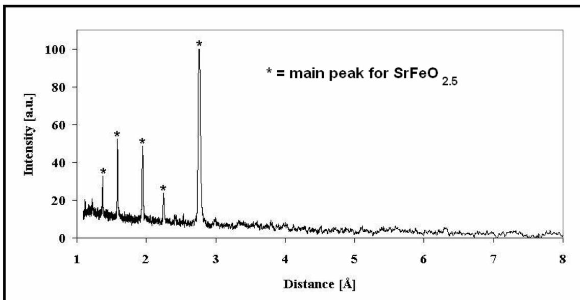
Fig. 5. X-ray powder diffraction data of the sample obtained by thermal decomposition of  $\text{SrNH}_4[\text{Fe}(\text{CN})_6] \cdot 3\text{H}_2\text{O}$  at  $900^\circ\text{C}$ .
