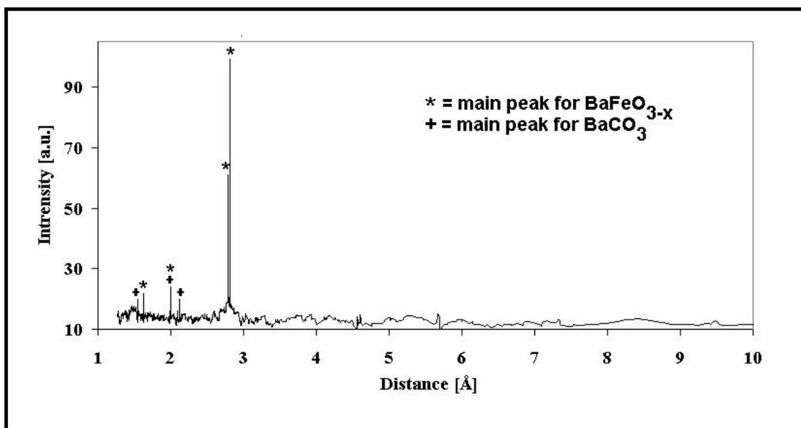
Fig. 6. X-ray powder diffraction data of the sample obtained by thermal decomposition of  $\text{BaNH}_4[\text{Fe}(\text{CN})_6]$  at  $900^\circ\text{C}$ .
