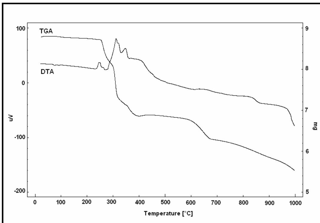
**Fig.4.** TGA-DTA curves of  $BaNH_4[Fe(CN)_6]$  in oxygen.
