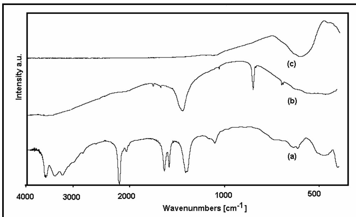
**Fig.1.** IR spectra for samples of  $\text{SrNH}_4[\text{Fe}(\text{CN})_6]\cdot 3\text{H}_2\text{O}$  at different temperatures: a) room temperature, b) 400 °C, c) 900 °C
