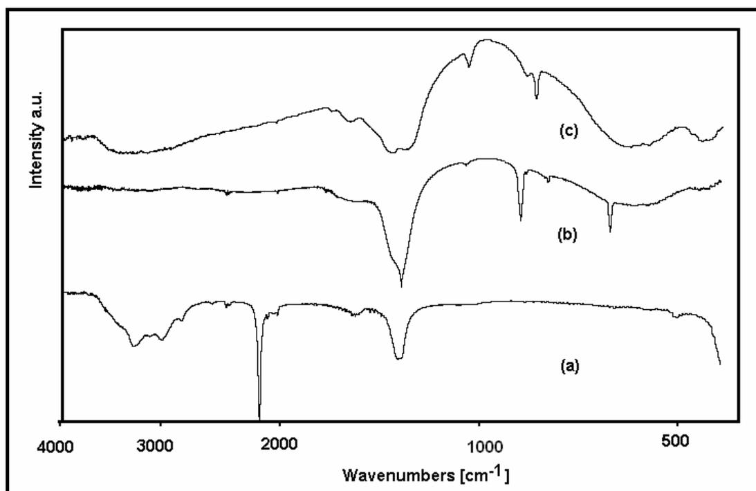
**Fig.2.** IR spectra of samples of  $\text{BaNH}_4[\text{Fe}(\text{CN})_6]$  at different temperatures: a) room temperature, b) 500 °C, c) 900 °C.
